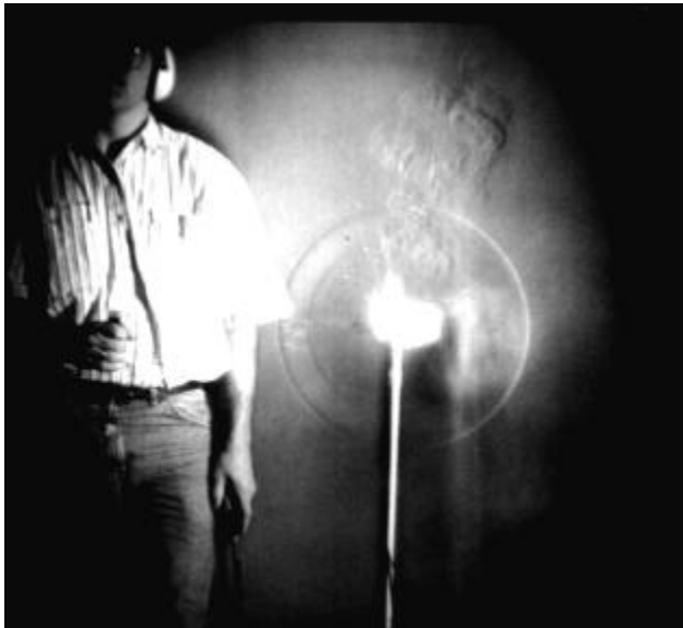
Figure 2. Single-Exposure Schlieren Image of Spherical Shock Wave from “Penny Firecracker”
