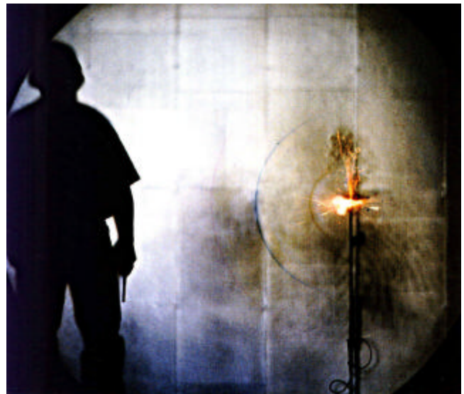
Figure 3. Color Triple-Flash Image of Spherical Shock Wave from “Penny Firecracker”
