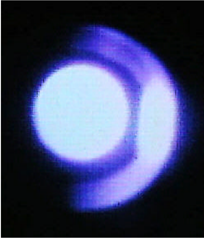
Figure 8. Ultraviolet image of plasma cutting viewed directly along the plasma jet axis from below the plate.
