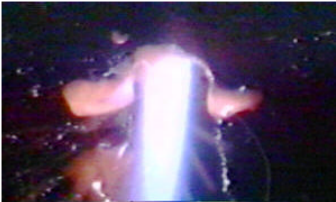
Figure 11. Image of a plasma cut with dross formation on a heavily-corroded workpiece, viewed from below leading the torch.
