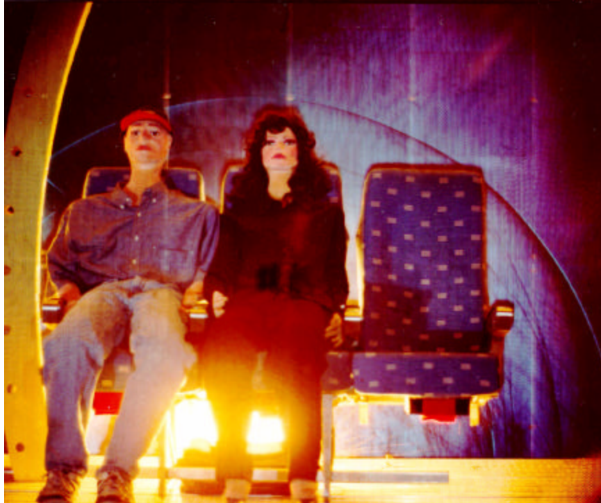
Fig. 3. Front view of an under-seat blast in the mockup aircraft cabin.
