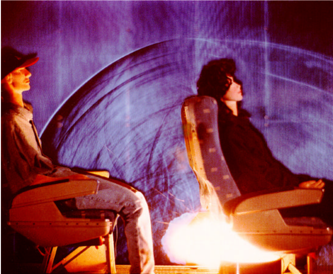
Fig. 2. Side view of an under-seat blast in the mockup aircraft cabin.
