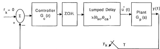
Fig. A.1 Lumped delayed control system
