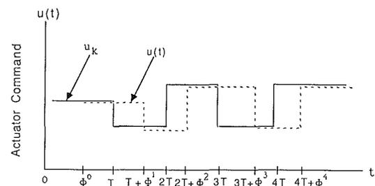
(a) Comparison of delayed and undelayed output
