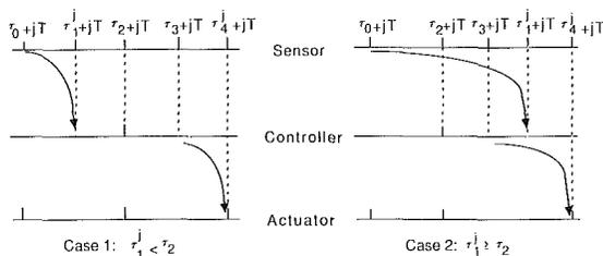
Fig. 3 Timing diagram for message transactions
