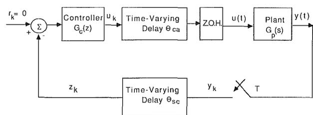
Fig. 2 Delayed control system
