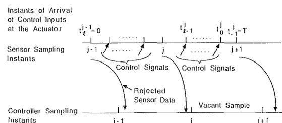
Fig. 4 Timing diagram for sensor and control signals
