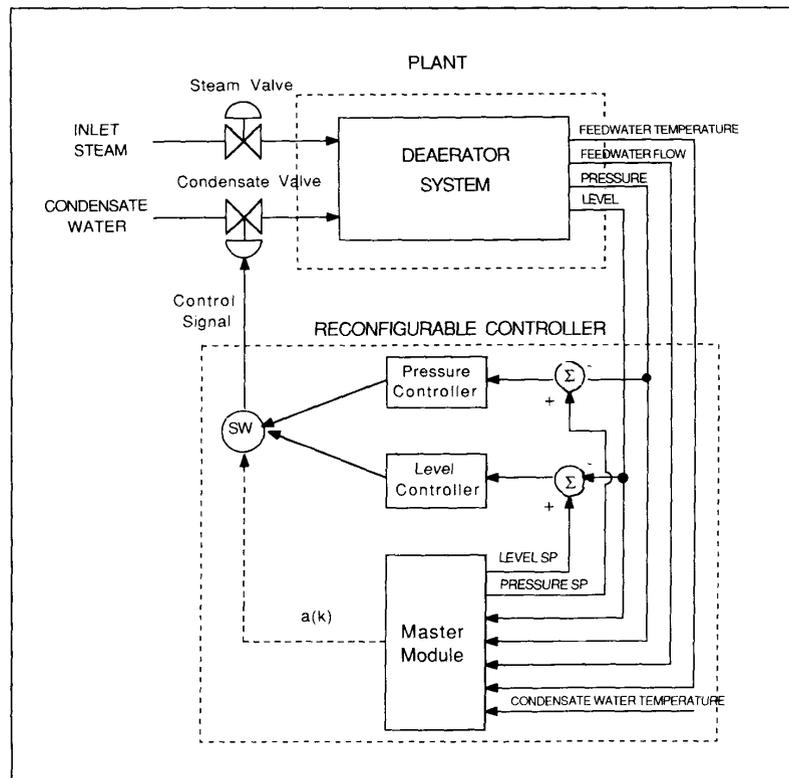
Fig. 1. Reconfigurable control scheme of the deaerator.
