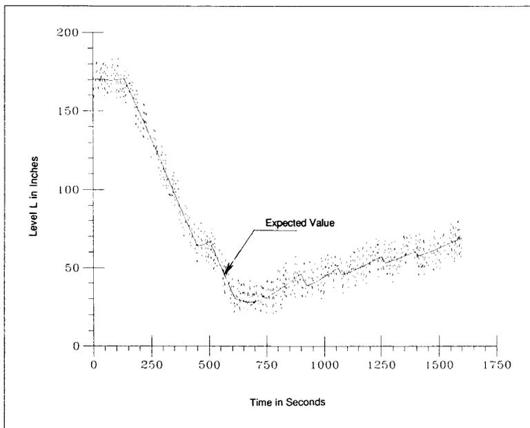
Fig. 8. Deaerator level transients using the reconfigurable scheme (with noisy measurements).
