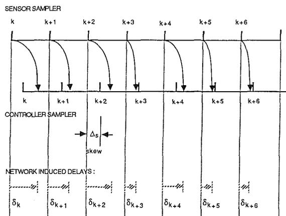
Fig. 1 Illustration of sensor to controller delay characteristics
