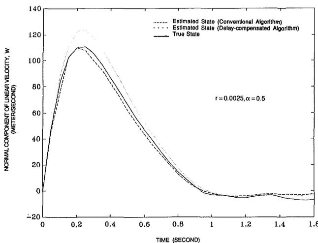
Fig. 3 Performance comparison of the state estimation algorithm [ $r = 0.0025, \alpha = 0.5$ ]
