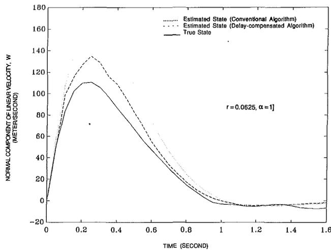
Fig. 4 Performance comparison of the state estimation algorithms [ $r = 0.0625, \alpha = 1$ ]
