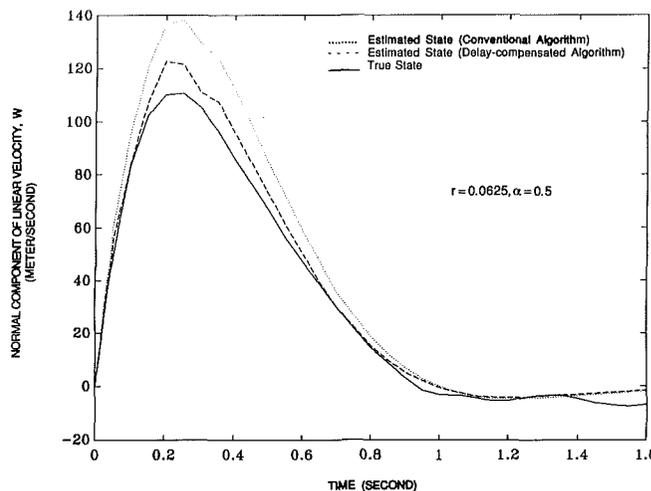
Fig. 5 Performance comparison of the state estimation algorithms [ $r = 0.0625, \alpha = 0.5$ ]
