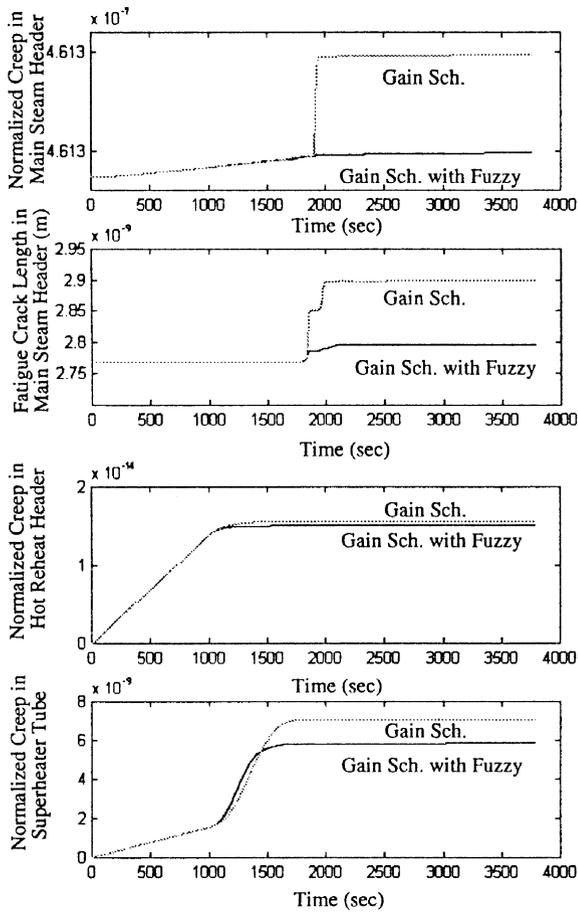
Fig. 11. Damage during ramp-down in the perturbed plant model.
