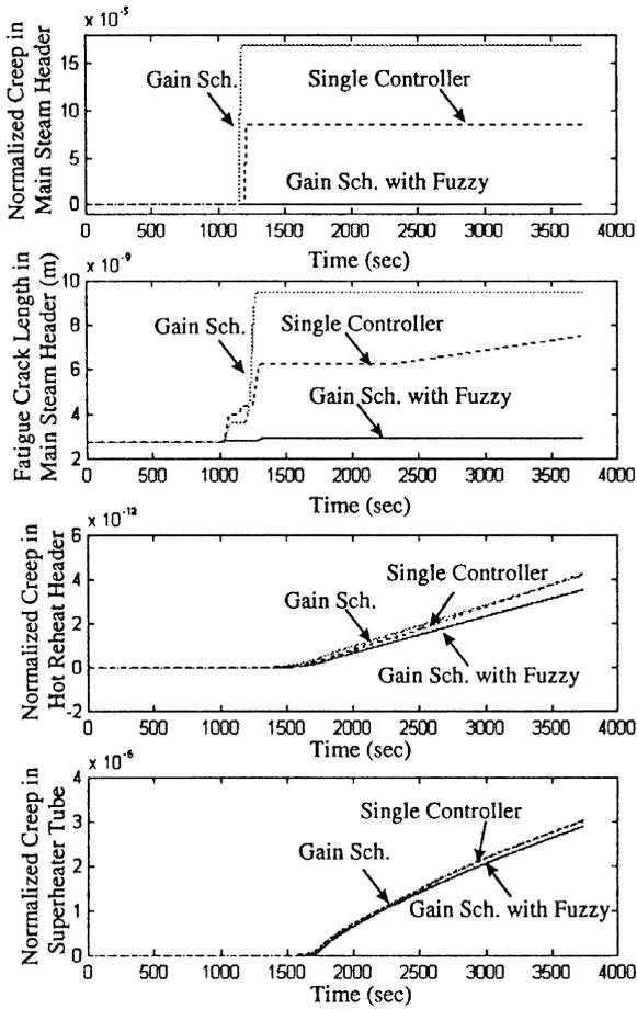
Fig. 9. Damage during ramp-up operation in the nominal plant model.
