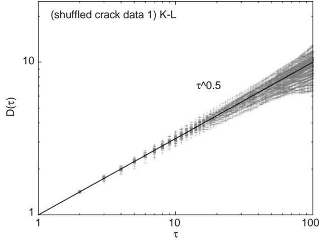
Fig. 5. SDA for the residual part of the KL decomposition after shuffling of the increments  $\{\theta_i\}$ . Note the random scaling of  $H \approx 0.5$ . The data refer to set #1 and the comparison has to be made with Fig. 4 (crack data 1) KL.
