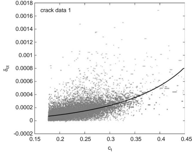
Fig. 3. Increments  $\delta c_t$  against crack length  $c_t$  fit with Eq. (8) (solid curve) for the experimental data of 7075-T6 aluminum alloy for the set #1:  $\Omega\Delta S^m = 0.0019 \pm 0.0002$  and  $m = 4.0 \pm 0.2$ .
