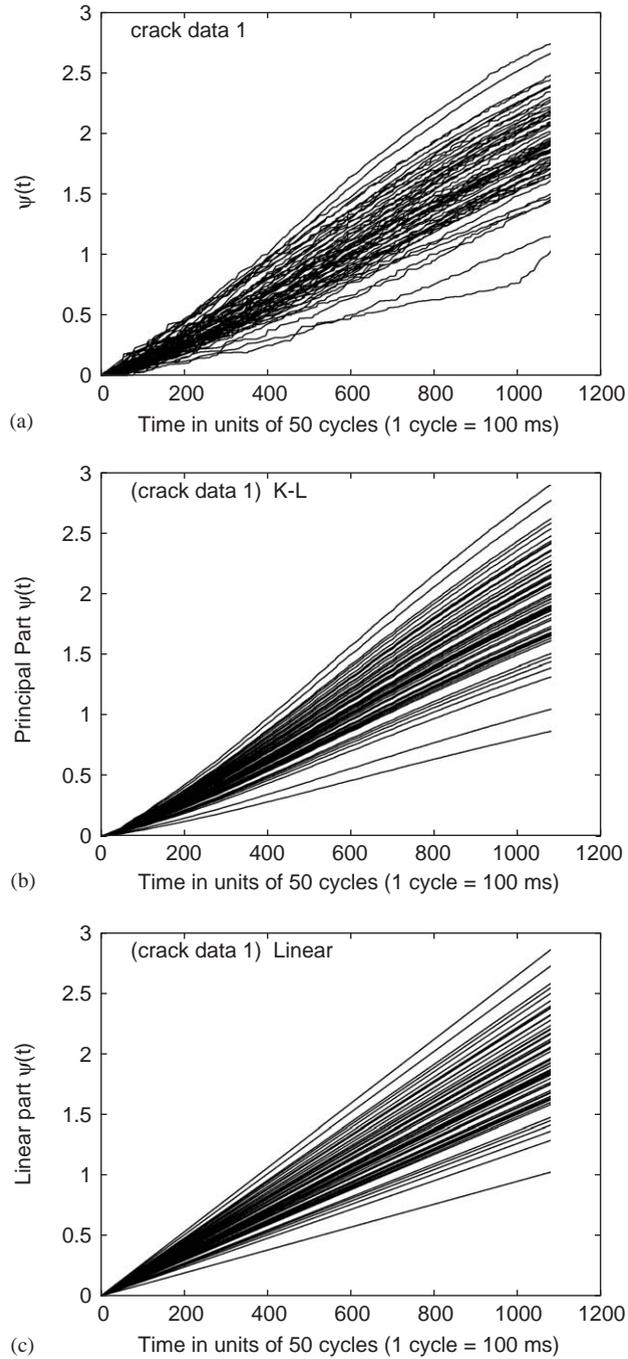
Fig. 2. (a) Curves  $\psi(t)$  obtained with Eq. (12) for the experimental data of 7075-T6 aluminum alloy for set #1. The value of  $m$  used is  $m = 4.0$ . (b) Principal part of the KL decomposition against (c) the linear approximation of the continuous model made in Eqs. (23) plus (24) of the curves  $\psi(t)$ .
