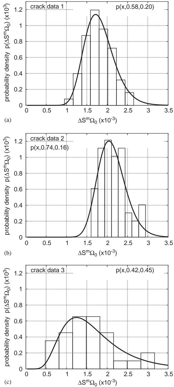
Fig. 7. Histogram of the quantities  $\Delta S^m \Omega_0$  of the continuous model of the experimental data presented by Eq. (25). The histograms are fitted with a lognormal distribution  $p(x; \mu, \sigma)$  shown in Eq. (29).
