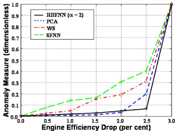
Fig. 2 Comparison of Different Methods of Anomaly Detection
