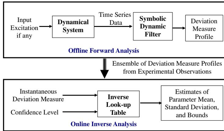
Fig. 1. Schematic diagram for symbolic dynamic filtering (SDF).
