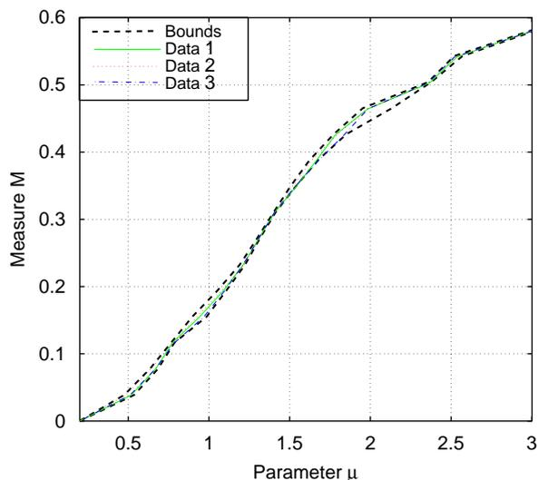
Fig. 9. Confidence intervals and test results for the van der Pol system.
