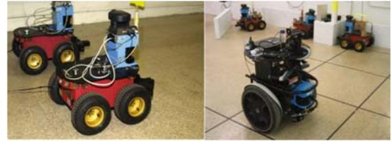
Fig. 5 The robot hardware: Pioneer 2AT and Segway RMP
