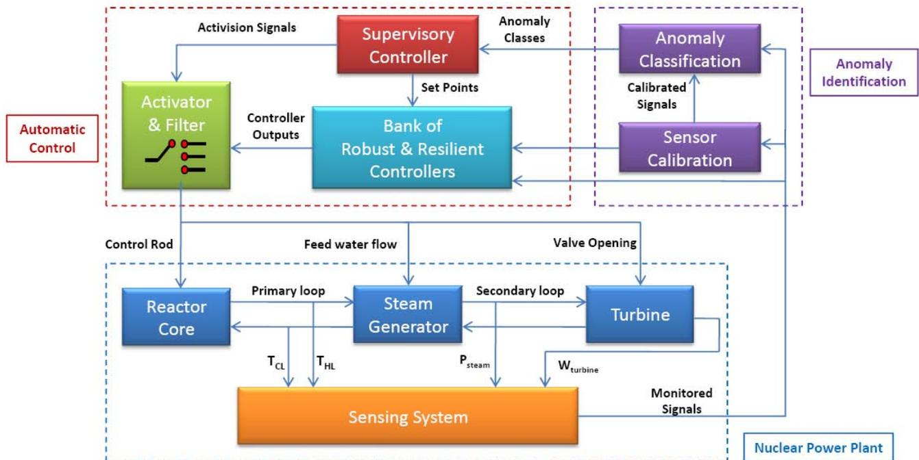
Fig. 1. An integrated scheme for anomaly identification and automatic control of nuclear power plants.
