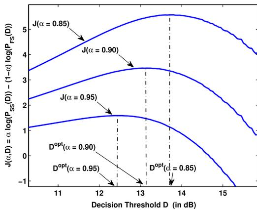
Fig. 3. Effect of threshold on the objective  $J(\alpha, D)$  for the track in Fig. 2.
