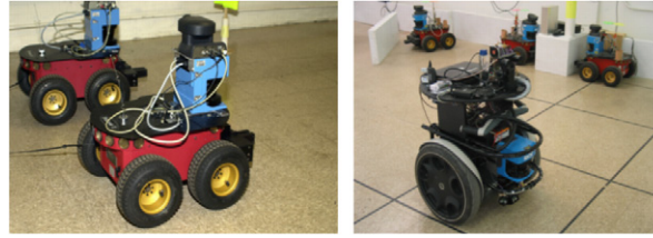
Fig. 5. Robot hardware: Pioneer 2AT (on left) and Segway RMP (on right).
