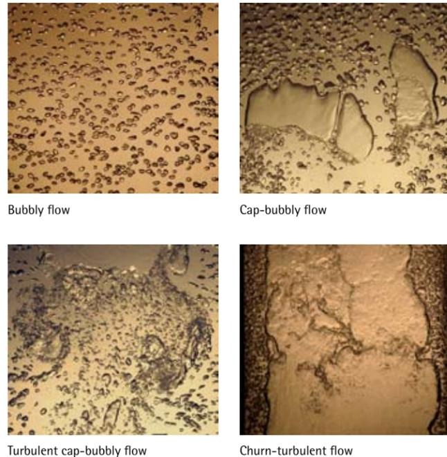
Figure 1. Different types of bubbles and interfacial structures in various two-phase flow regimes. Images are captured from air-water two-phase flow in rectangular flow channel.
