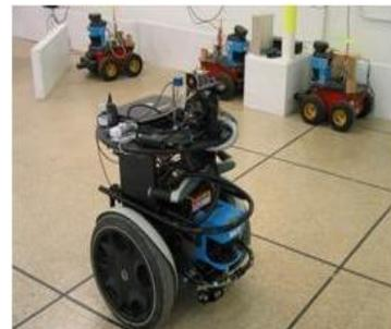
Figure A-4 Team of Segway and Pioneer 2 AT Robots
