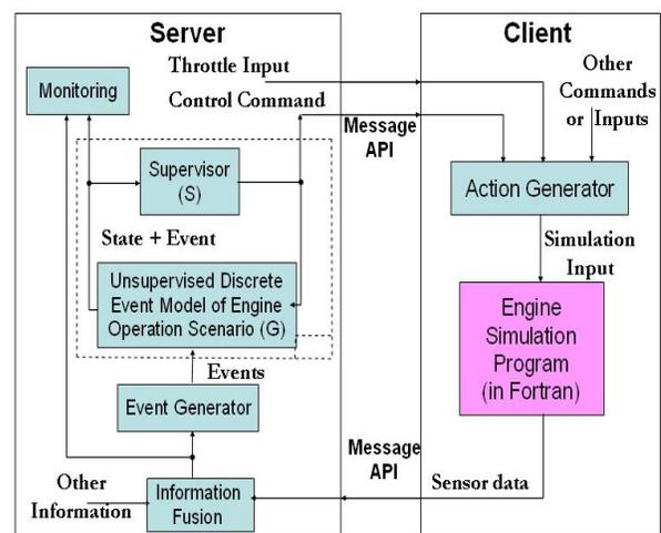
Figure A-8 Discrete Event Supervisory Control of Gas Turbine Engines
