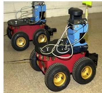
Figure A-3 Pioneer 2 AT Robots
