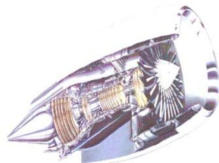
Figure A-6 Typical Gas Turbine Jet Engine
