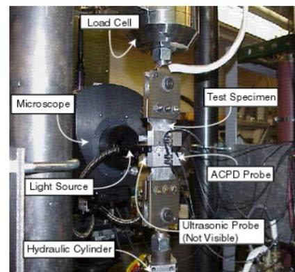
Figure A-1 Fatigue Damage Apparatus
